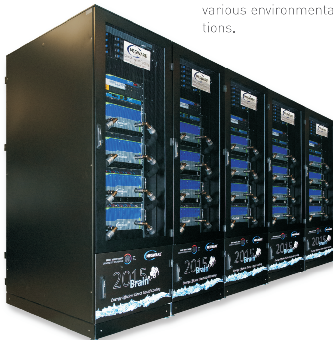
Fig.: Example of a ColdCon system with direct water-cooled compute nodes at the University of Greifswald
